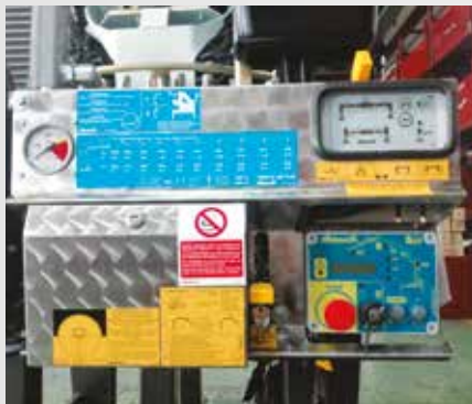
Comandi accessibili da terra. Tutti i carter in acciaio inox AISI 304. Controls can be reached standing on the side. All the carters are in stainless steel AISI 304. Commandes accessibles de terre. Tous les carter sont en acier inox AISI 304. Von der Seite steuerbar. schutzplatten in Edelstahl AISI 304.
