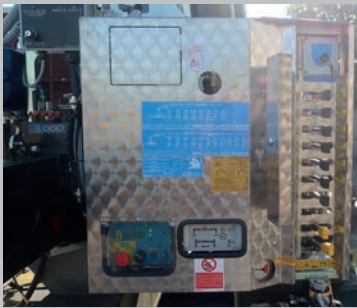
Comandi accessibili da terra. Tutti i carter in acciaio inox AISI 304. Controls can be reached standing on the side. All the carters are in stainless steel AISI 304. Commandes accessibles de terre. Tous les carter sont en acier inox AISI 304. Von der Seite steuerbar. Schutzplatten in Edelstahl AISI 304.
