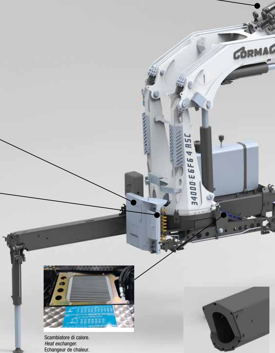
Comandi accessibili da terra. Tutti i carter in acciaio inox AISI 304. Controls can be reached standing on the side. All the carters are in stainless steel AISI 304. Commandes accessibles de terre. Tous les carter sont en acier inox AISI 304. Von der Seite steuerbar. Schutzplatten in Edelstahl AISI 304.
